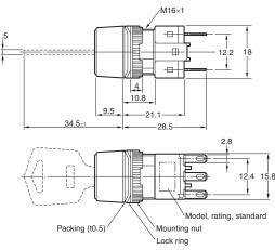
Dimensions • The Dimension shows 2-switch outputs. • The lamp terminal is also provided with non-lighted models. • A rectangular model is listed as an example. (Unit: mm)
